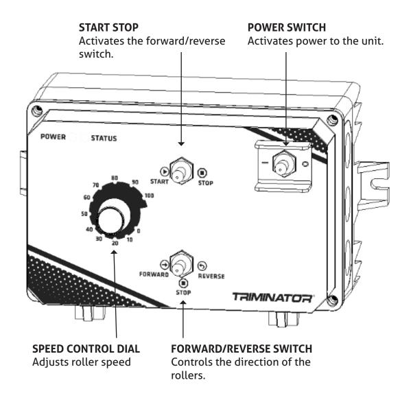
NOTICE: The BuckMaster series offers redundancy controls for safe operation. In order to operate all controls must be in an active position and the emergency stop must be in an operating position.
