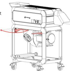
Position the circular mouth of the trim bag over the outlet of the fan housing, and cinch the drawstring around the raised lip to secure the bag to the machine.
