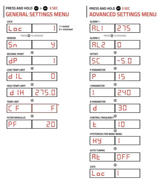
**NOTICE** Make sure your Temp Unit is set to Fahrenheit. Setting Fahrenheit temps in Celsius can result in melting components of the machine.
